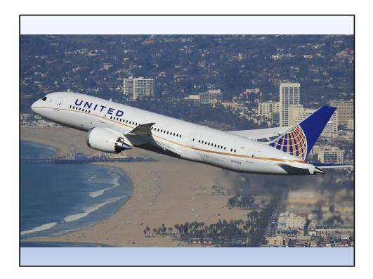
This aircraft, the Boeing 787 Dreamliner is also powered by two of the General Electric GEnx engines. The Rolls Royce Trent 1000 engine can also be fitted to this aircraft. Note that this aircraft, like many new airliners, only has two engines. This gives a large saving in the cost of engines but, as we will see, brings other problems in designing these aircraft.
