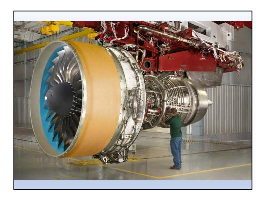
This is one of the engine types that the customer can choose to power the Airbus A380. This is the Engine Alliance GP 7200, the other possible engine is the Rolls Royce Trent 900. Both of these engine types can produce up to 70,000 lb of thrust.
