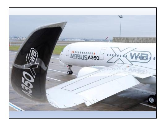
This is the latest large airliner from Airbus, the A350XWB. This is also a twin engine aircraft and again the engines have to very powerful to allow it to continue to take-off safely after an engine failure.
