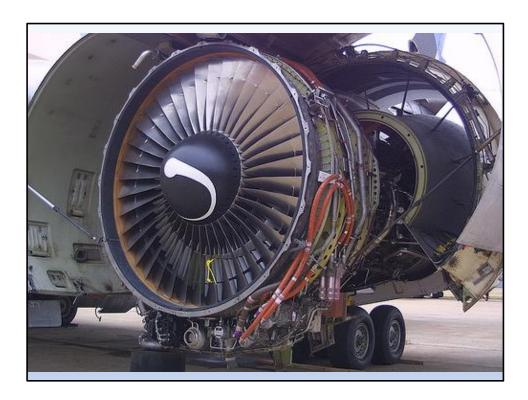
This is the General Electric CF6-50 engine, one of the most common of the big turbofan engines. In this photo the cowlings have been opened up to allow the engine to be inspected. We can see the size of the fan and the number of blades. The odd white shape on the spinner is to make the engine face more visible to let birds see it coming and hopefully avoid the engine.
