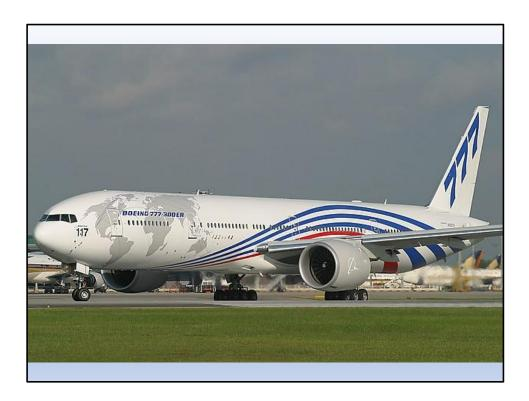
This big modern airliner, the Boeing 777-300ER, needed a really powerful engine. So the challenge for the engine designers was to design an engine that could produce more than 100,000lb of thrust.
