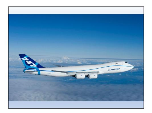
This is the latest in the long line of types of the Boeing 747 aircraft. The aircraft familiarly known as the Jumbo Jet. This is the Series 800 and is powered by four of the General Electric GEnx engines that can produce up to 76,000 lb of thrust.
