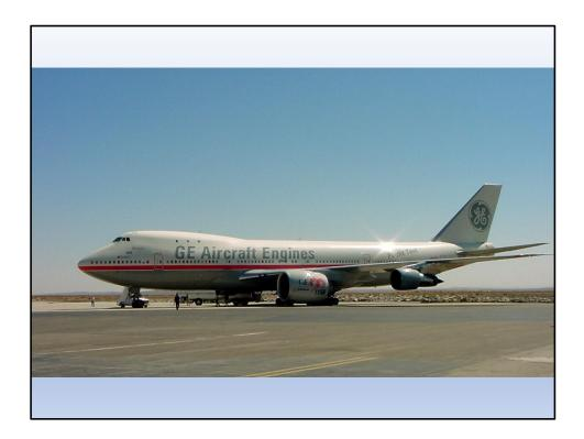
This is the GE90-115B being flight tested on GE's test aircraft. It is mounted on the left-hand inboard engine pylon and you can see how large it is compared to the existing engines.
