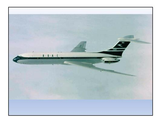
This is the beautiful Vickers VC10 and it was powered by four RR Conway engines. It set speed records for crossing the Atlantic back in the 1960's and 70's. The aircraft was capable of cruising at 580 mph which was getting very close to the speed of sound at its cruising altitude.
