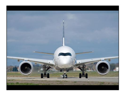
As aircraft became bigger, heavier and faster there was a need for even more thrust. The impellers became much bigger and were now commonly called fans. You can see the fan inside the cowlings of this Airbus A350 airliner.
