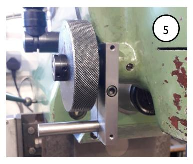
Something had to be done. The first idea was a sliding collar which would fit over the spindle and lock to it. It would then touch the head body when the appropriate depth had been reached. This would need a series of gauge blocks to set it to the correct height on the spindle. However, no graduated scale would be available and the guard would also still have to be removed and so this idea was rejected.
