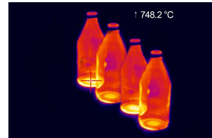
Hot spot detection in glass bottle production
