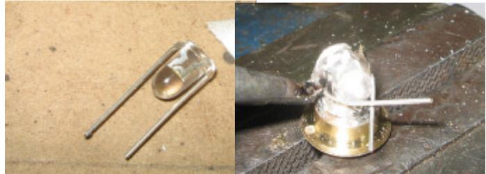
*The LED bent ready for soldering, left, and being soldered, right.*
