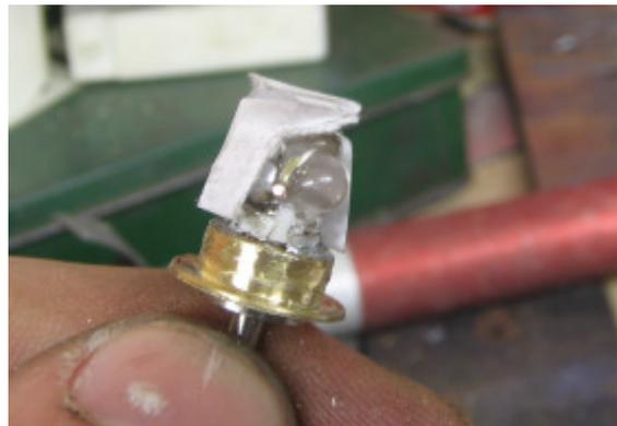
*Complete with paper insulation ready to go into the lamp.*
