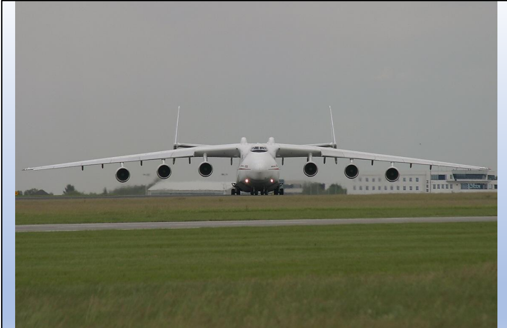
The huge 600 ton Antonov An225 is the heaviest aircraft in the world. Designed to cruise at 500 mph at 35,000 ft carrying a load of 245 tons
