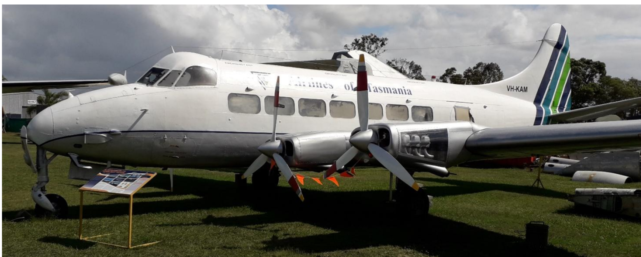
Nothing too unusual about this one – it is de Havilland Heron, VH-KAM once operated by Airlines of Tasmania. Look again though. The type never left the Chester factory with flat-six Lycoming engines. This example has an interesting history, including some service in the UK with Morton. It lost its Gipsy Queen engines in 1975, and I do like the sleeker appearance.
