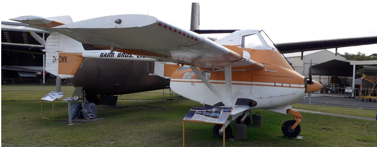
ZK-CWX is an example of the Australian designed and built, Transavia PL-12 Airtruk agricultural aircraft. Powered by a 300hp Continental IO-520, six cylinder engine, the type could hardly be more different from the Starship above.
