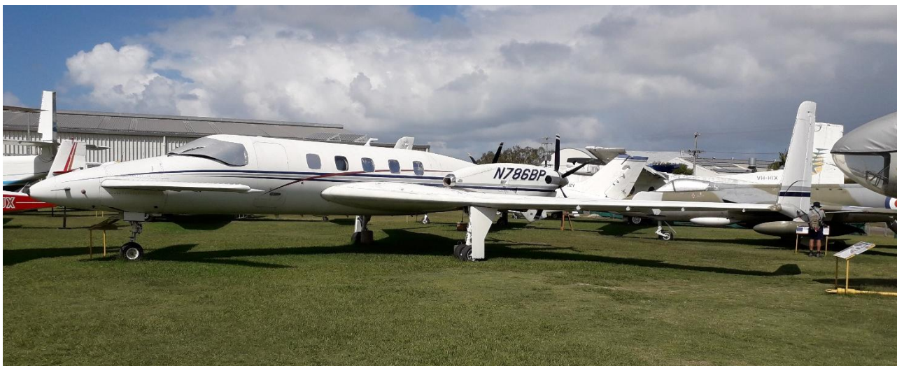
The Bert Rutan-designed Beech Starship was a radical corporate type when introduced during the 1980s. A canard configured, twin turboprop pusher design, only 53 were built. Always short on performance, eventually Beech pulled the plug on the type in 2003. QAM's example is N786BP.
