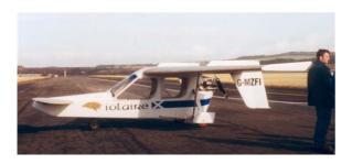
"Iolaire" is the only one of Hugh's aircraft to actually leave the ground - it has around 20 minutes on the clock. Noteworthy (and particularly controversial) is the use of an "all-flying" canard for pitch control.
