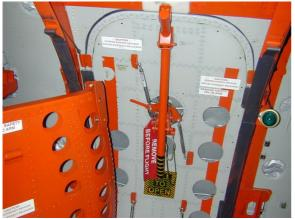
BAE SYSTEMS' photograph of the installation described in the article. Clearly visible are the large, central pull handle and to left, part of the air dam that is fired out of the open door. If anybody has access to a picture of the door fully deployed, we would be happy to publish in a future newsletter
