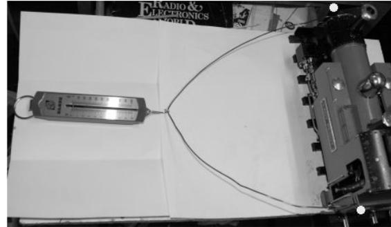
The spring balance was connected to a higher fixing point and a measurement made.
