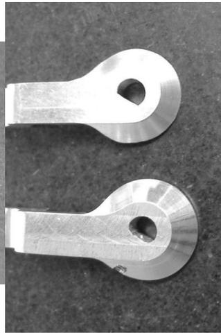
Pictures here show the Push-Broach (supplied by WDS MARLCO) and the lever before and after broaching.
