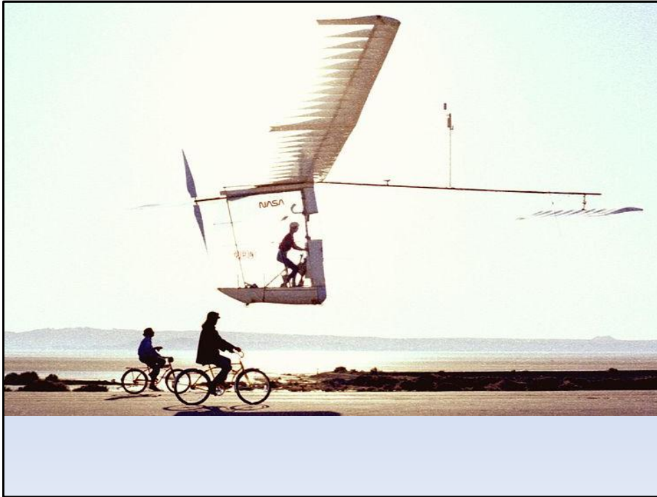
The Gossamer Albatross man-powered aircraft was pedalled across the English Channel in 1979. Note the relatively small forward wing. This extremely light aircraft flew at about 10 mph.
