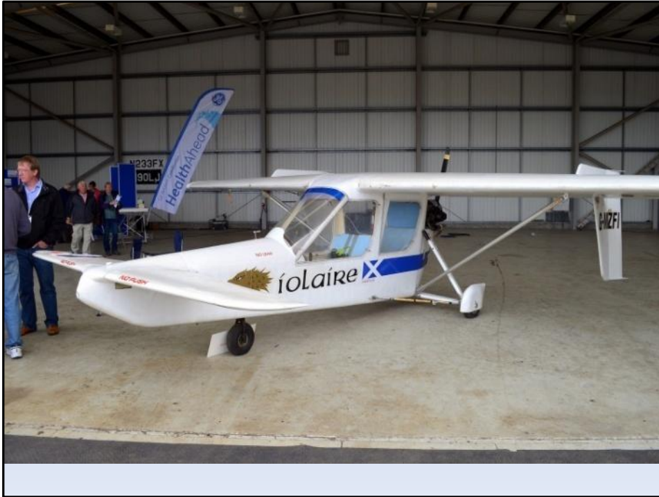
Hugh Lorimer, an Ayrshire school teacher, designed and built this aircraft called the Iolaire [the Eagle]. It has a horizontal stabiliser at the front and two vertical stabilisers at the back.
