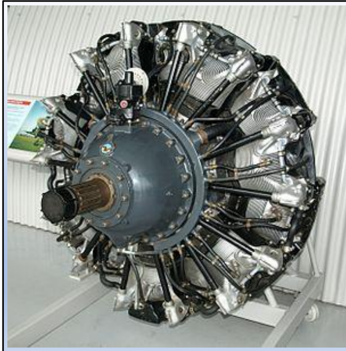
The Pratt and Whitney Twin Wasp Engine
