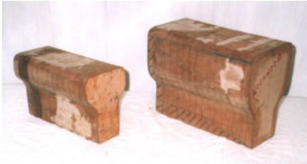
To save time, a start was made on the plate formers. Slices of MDF were cut to build up the two wrapper formers with small irregularities being smoothed out with car body filler. End plate formers were made in the usual way – 1/8" thick mild steel attached to plywood backing with wood screws. The Belpaire throatplate proved to be a challenge as it is double flanged, as shown in the photo. About 5/8" was allowed for forming each flange, and a hide mallet used
