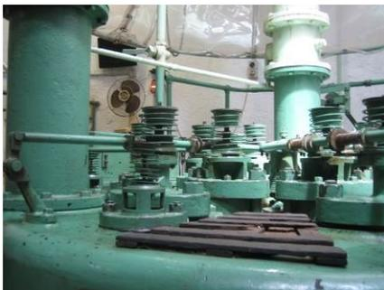
*This is the top of the valve set with outside spring. These are so soft that they can be pushed down with one finger*
