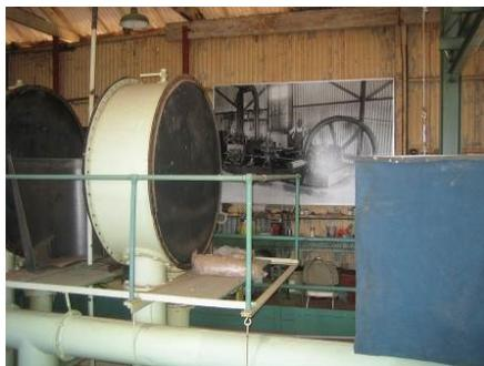
*This is the gas bag which feeds the cylinder from the gas making (from coke) plant outside the main building*
