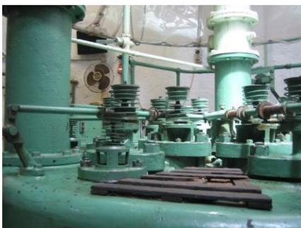
*This is the top of the valve set with outside spring. These are so soft that they can be pushed down with one finger*
