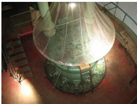
*The gas exhauster shield above the main valve work*
