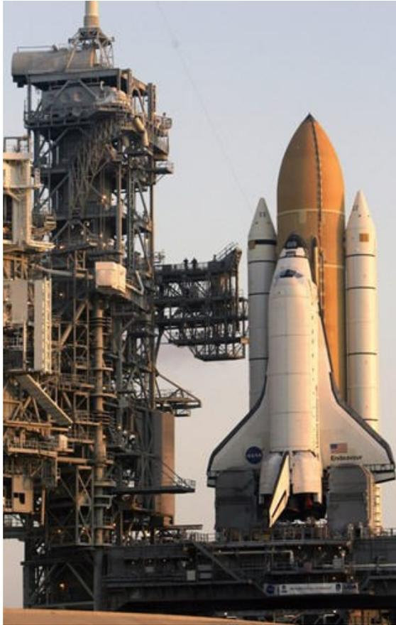
The engineers who designed the SRBs would have preferred to make them a bit fatter, but the SRBs had to be shipped by train from the factory to the launch site. The railroad line from the factory happens to run through a tunnel in the mountains, and the SRBs had to fit through that tunnel. The tunnel is slightly wider than the railroad track, and the railroad track, as you now know, is about as wide as two horses' behinds.
