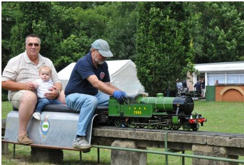
John Eldred of Welling visited with his V3 2-6-2 tank “Enterprise”. Taking six years to build it was completed in 2009. A good, powerful 3 cylinder loco—if only the A1 group would build a full size version as rumoured. John has lent out the boiler templates for his loco, and so far 4 boilers have been completed using them, including that of Tom Parham’s Enterprise.
