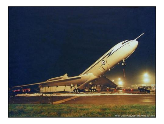
The nose wheel of this Royal Air Force Vickers VC-10 transport should be on the ground. This incident occurred during maintenance when the aircraft was being de-fuelled prior to some work to repair leaks in the fuel system.
