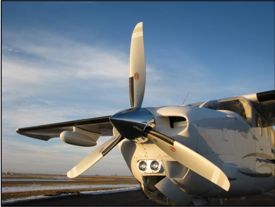
This photo shows a typical variable pitch propeller on a light aircraft.
