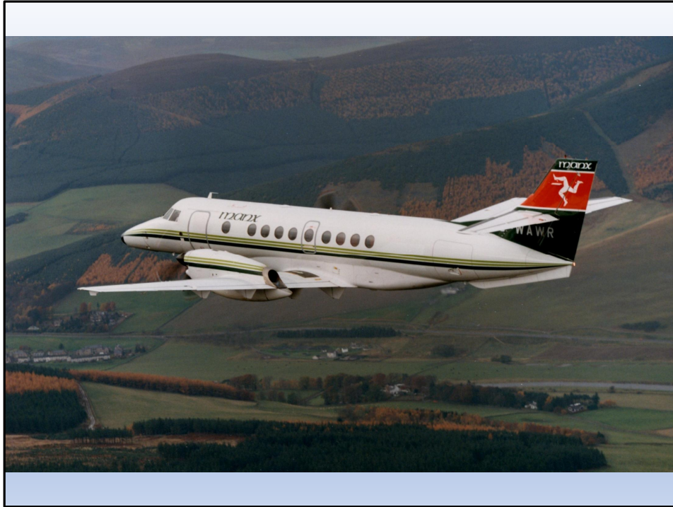
This Jetstream 41 aircraft, also built at Prestwick, has its horizontal stabilising surface mounted halfway up the vertical stabilising surface.
