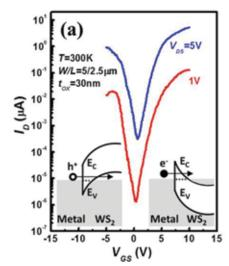
Figure 21. The drain current as a function of the gate voltage at different values of the gate voltage VGS indicates ~105x on/off ratio. The scheme presents an electron and hole conduction
