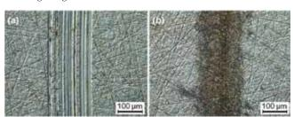
Figure 19. Optical micrographs of wear traces left on a steel disc after 100 m of sliding of a steel ball. The ball was lubricated with (a) pure PAO base oil, whereas in (b), 5 wt.% of MoS<sub>2</sub> nanotubes have been added to the lubricating oil.
