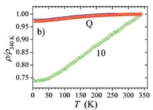
Figure 1: Anisotropic electrical resistivity of a decagonal quasicrystal d-Al-Co-Ni, measured
