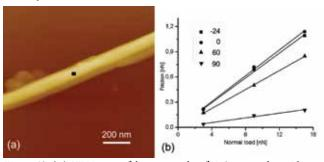
Figure 18. (a) AFM image of the topography of MoS<sub>2</sub> nanotubes with a diameter of 170 nm. The scanning force was 3 nN, the scanning region is indicated with the square. (b) Friction force for different directions of scanning along the nanotube.
