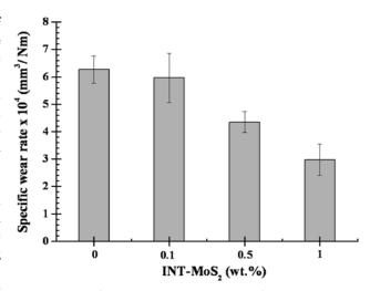
Figure 20. Wear of pure iPP and nanocomposites of iPP and MoS, nanotubes.
