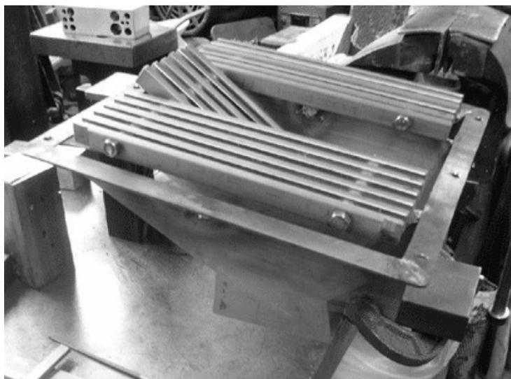
Four radiant super heaters have been constructed, and the boiler cladding is being assembled. Also the cab and running plates are in hand.
