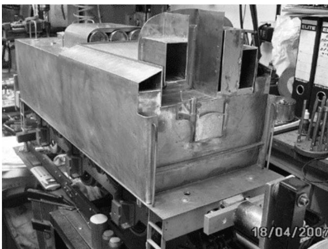
2001. Main frames, bogie and tender frames water cut to profile as per M.E. drawings. All chassis stays bent and formed on ally formers. Outside motion brackets, outside guide bar brackets etc. All parts hand profiled (each 25-30 pieces) in every case to suit brazing. Assembly fixtures made in each instance. Each unit was No.2 Silver Soldered in one hit on fixtures, sand blasted and primed.
