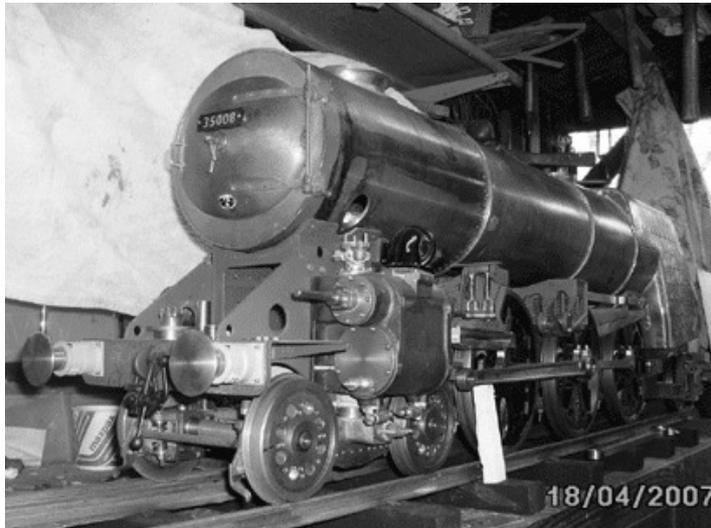
Rebuilt Southern Railway Merchant Navy's are similar to "Brits", which borrowed much from Bulleid's design. I knew 'Ariel' would be a complicated loco to build and would test all my skills, and it certainly has some. As the full-size was an all welded design and manufacture, the model has tested my ingenuity to make the 1/12 scale version look 'welded', if you see what I mean.
