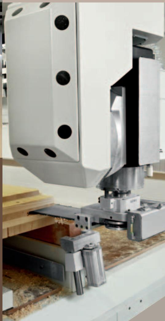
With the aggregate "motor-saw" are produced faster opening angles of 90 ° and deep grooves on all sides of the wall.
