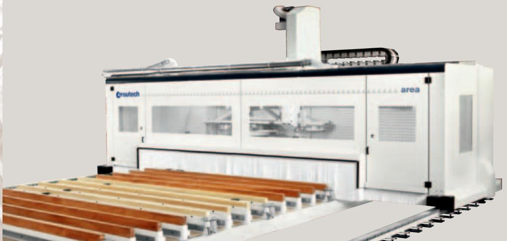
The solid and robust structure moves on rails precision low vertical profile to ensure high standards of accuracy and allow the operator easy access to climb over the work area with ergonomics.
