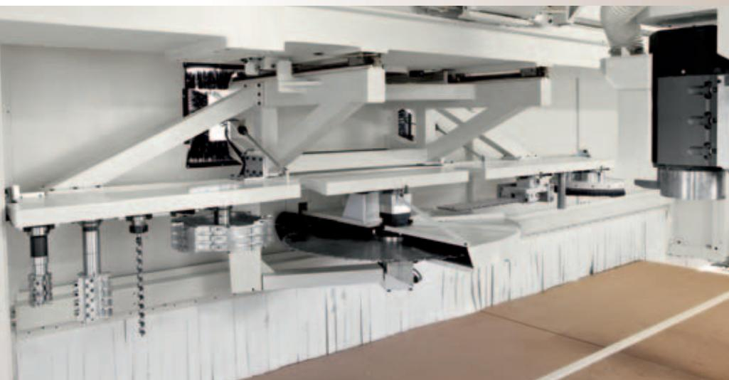
The magazine at 12 stations has been designed to accommodate all the tools needed to complete the entire working cycle. Anchored to the mobile gantry allows to have on board always the right tool to speed up execution of the entire workpiece program.
