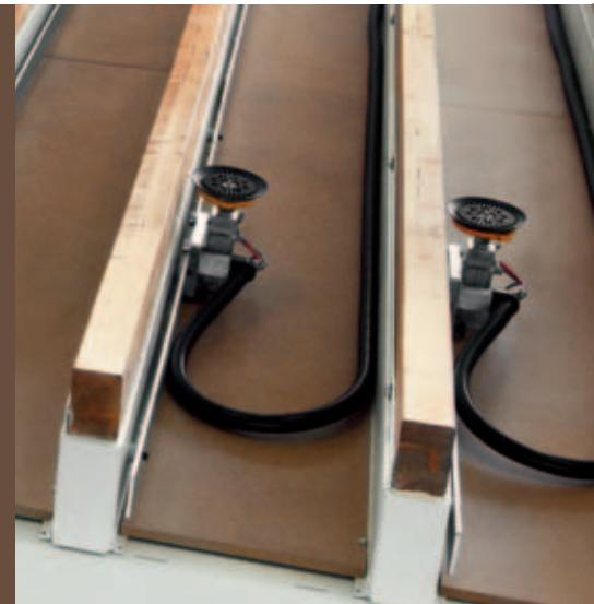
▲ The vacuum system allows the use of vacuum suction cups automatically activated to stop small workpieces with small surfaces.
