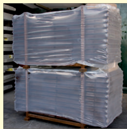
COMPOSITION PALLET pallets to be returned (doors without coverings, without cardboard) for delivery to a single customer, max optimization, 11 doors + 11 doors. Its possible to place up to 4 pallets one on top of the other. Idimensions 120x220xh114 cm total weight with 11 doors without covering 0,50 tons.
