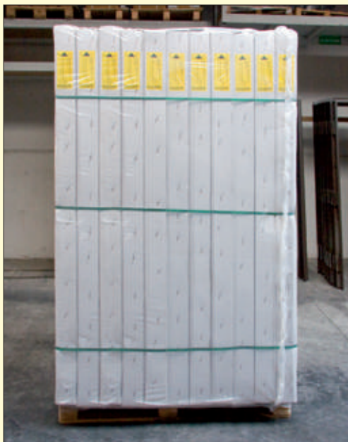
VERTICAL COMPOSITION PALLETS 11 covered doors total weight 0,90 tons dimensions 120x106xh238 cm; 20 door frames total weight 0,30 tons dimensions 120x105xh233 cm.
