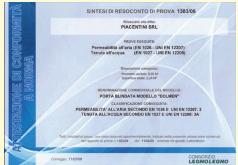
Air permeability class 2 and water resistance class 3A.
