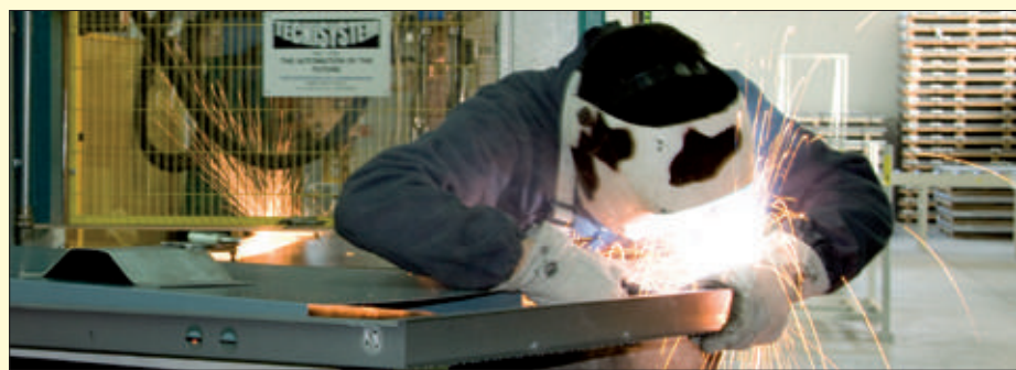
Welding of the door body.
