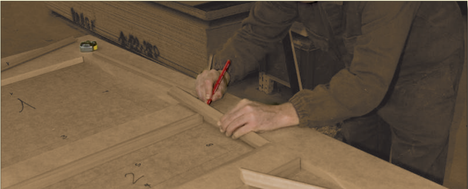
Processing of frame panel with relief surface.
