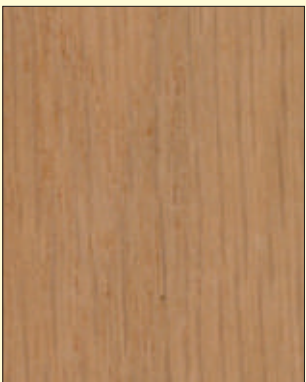
OKUMÈ veneered with Durmast natural lightly stained
