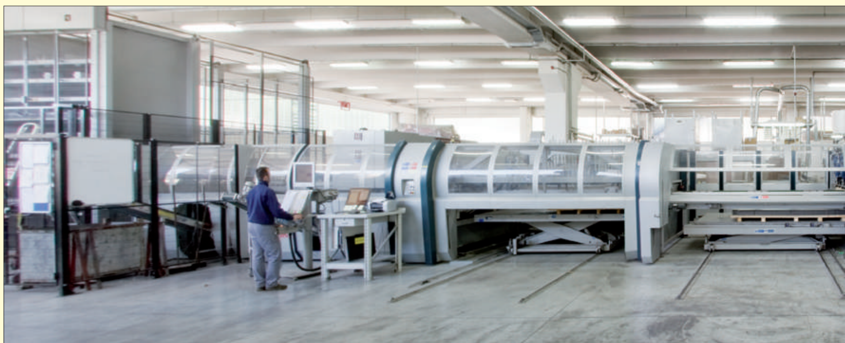
Salvagnini Automatic sheet metal line.
