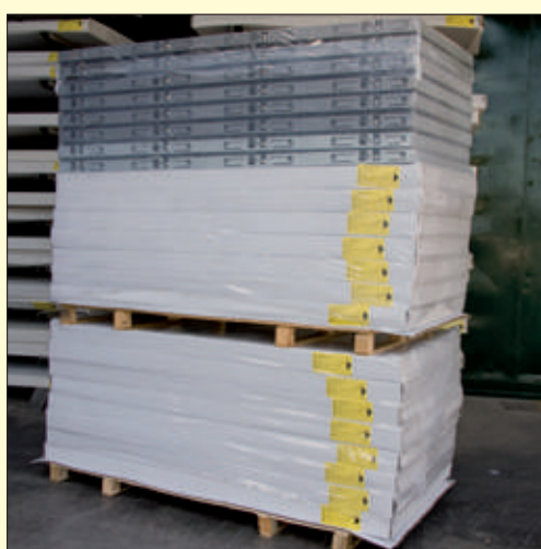
COMPOSITION PALLET (doors with cardboard) for delivery to a single customer, max optimization; 8 doors + 7 doors + 15 door frames. Total weight 1,4 tons ; package 110x220xh240 cm.
