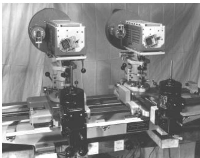
Rear view showing differential screw assemblies, cross slide motors and gearboxes and the special rule and two verniers. (The cameras were the smallest made by Pye Ltd., which by today's standards were large and quite heavy.)
