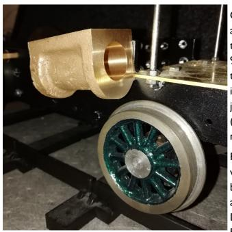
Onto the bore, spotted as before and drilled through in stages up to 9mm. Big enough for the boring head. Slowly in 5 thou cuts up to just shy of a whopping (and here comes point no 1) 11/16ths bore.
