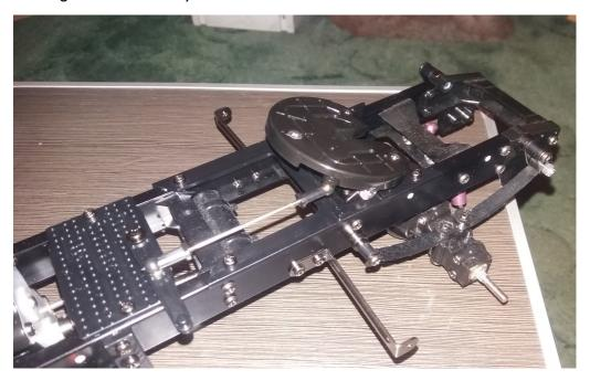
Next I continued with the fifth wheel assembly complete with release lever and fitted it to the chassis.
