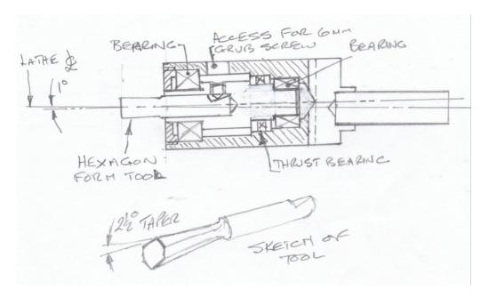
High speed tool steel would be better but I don't have a cutter grinder!
